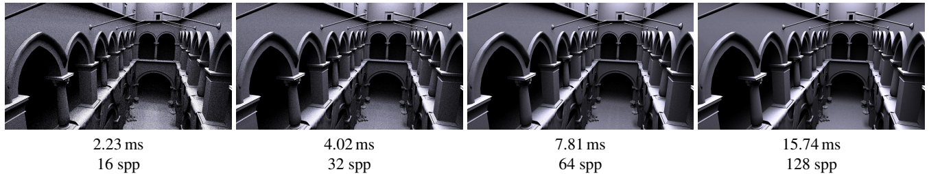
Figure 8: Comparison of the rendering results without textures in the Crytek Sponza scene using different numbers of ray samples per pixel. From left to right: 16, 32, 64, and 128 spp.
