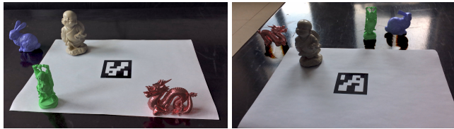
Figure 9: Reflections of virtual objects on the real scene with a non-diffuse BRDF.
